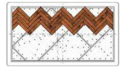
Lay out four or five rows of parquet in the same way as the first. Make sure that each row is laid out evenly and fits tightly against the previous one. Check regularly for proper installation and expansion gaps. Make sure that everything is flat.
