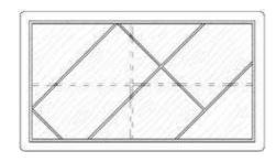
Install a second layer of plywood on top of the first layer, also made of entire sheets, but at an angle of 45° relative to the first layer. This will give to the whole structure additional rigidity, strength and stability.
