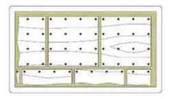
Additional fixation is provided by dowel nails or self-tapping screws, which should be installed at intervals of 15-20 cm along the edges and 20-30 cm in the center of each sheet. The fastening depth should be at least 30-40 mm to ensure reliable fastening of the plywood to the base.
