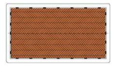
Continue laying to the opposite wall, remembering to install spacers along the walls. Once installation is complete, use the remaining pieces of parquet cut at the beginning. Clean the parquet from debris and dust using suitable care products.
